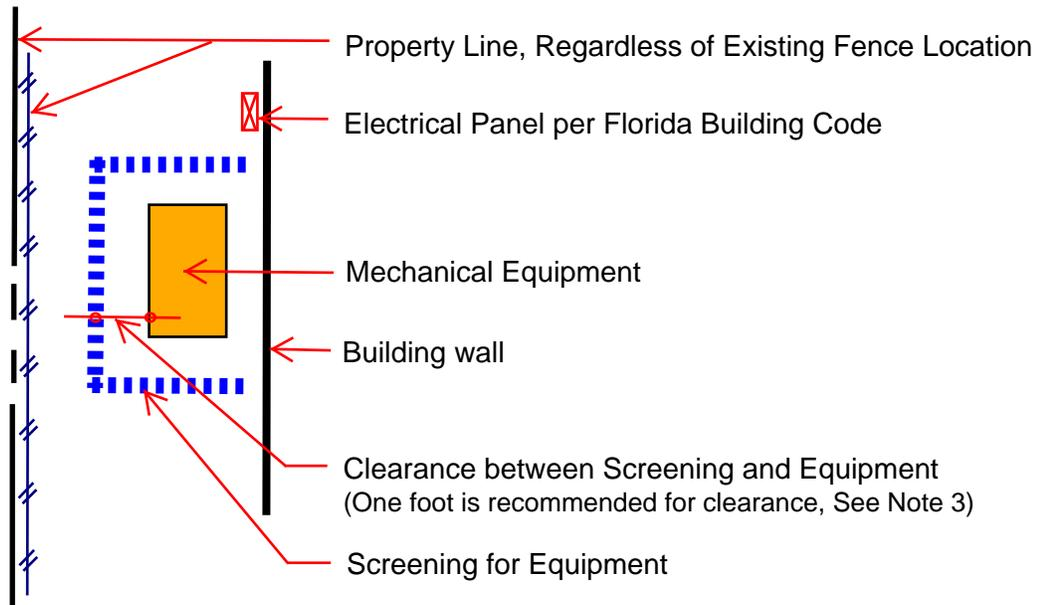
Per Code Section 155.5301.A.2.b, Ground-Mounted Mechanical Equipment shall be screened by **adjacent buildings, dense continuous hedges, or decorative walls or fences.**
