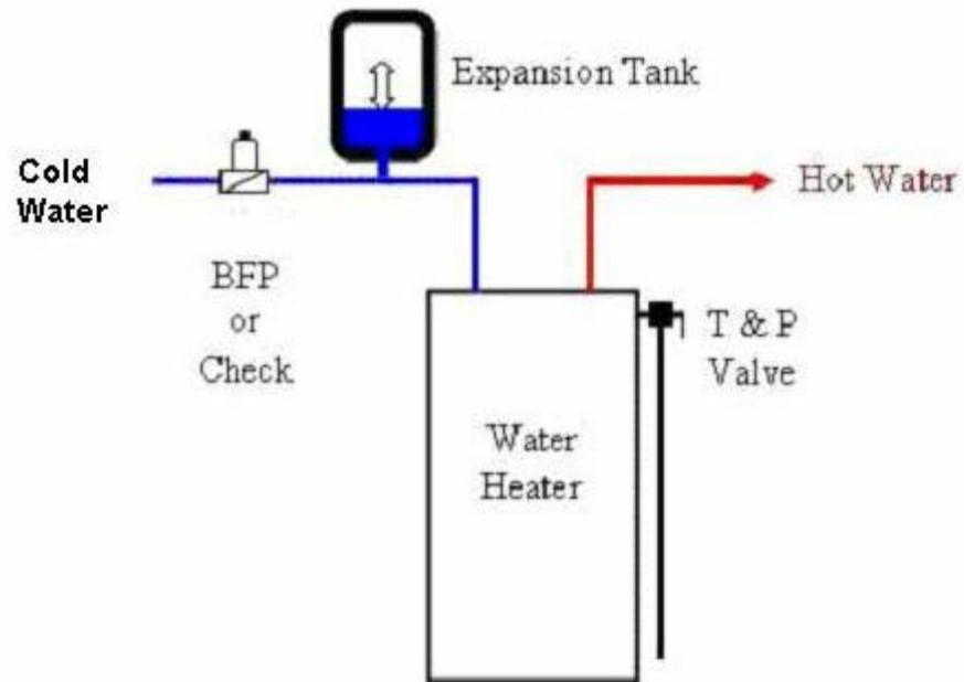
Another method of controlling thermal expansion is by the use of a thermal expansion tank. This tank must be installed on the water supply as show in Detail B. Thermal expansion tanks must be properly sized and installed as per the manufactures installation instructions.
